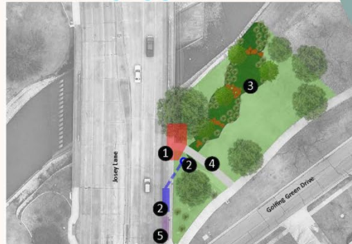
Left: Design for enhanced bus stop with water quality inlet & bioswale. Farmers Branch Conceptual Bus Stop Designs BGG project, 2020.
