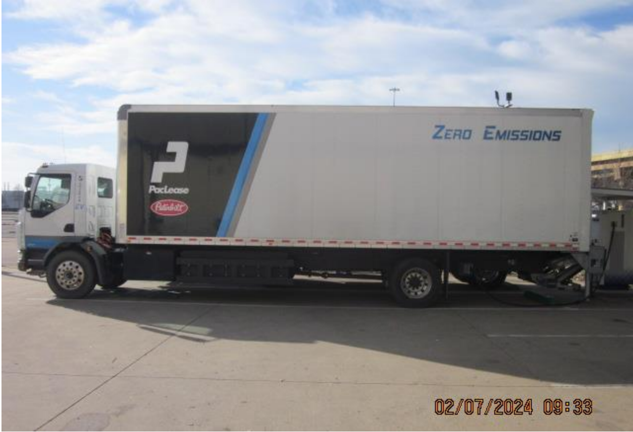
All-Electric Truck Side Profile Connected to Charging Unit
