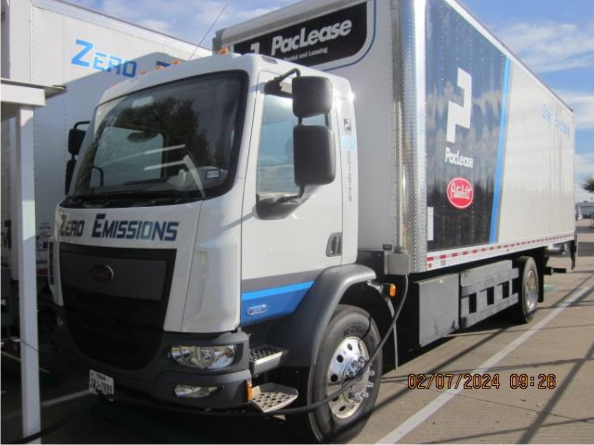
All-Electric Truck Front and Side Profile Connected to Charging Unit
