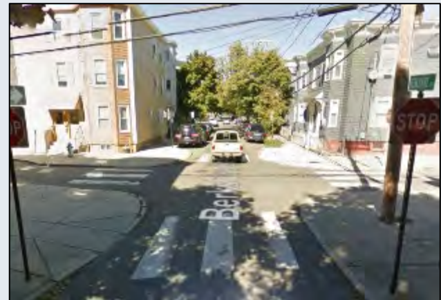
Motorist view of the curb extension at Berkshire and Plymouth Streets
