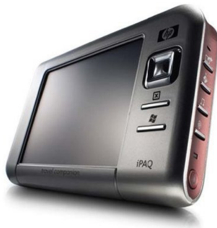
Figure 2-2: GPS-Enhanced Palm Device for On-Board Counts
