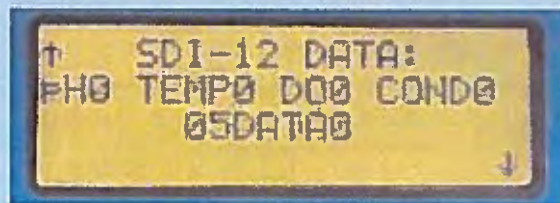
Display window showing SDI-12 connection status.
