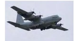
**C-130 Hercules** The C-130 Hercules primarily performs the intra-theatre portion of the airlift mission. The C-130 can be rapidly configured for various types of cargo, including palletized equipment, floor-loaded material, airdrop platforms container-delivery-system bundles, vehicles and personnel, or aeromedical evacuation. Currently, the eight C-130 Hercules aircraft stationed at NAS Fort Worth JRB are with the Texas Air National Guard's 136th Airlift Wing.
