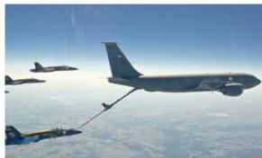
KC-135 Stratotanker The KC-135 is primarily an aerial refueling military aircraft; however, KC-135 variants serve as flying command posts, pure transport, electronic reconnaissance, and photo-mapping aircraft.
