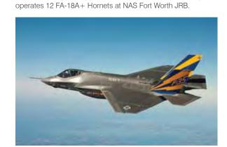
F-35 A/B/C Joint Strike Fighter, Lightening II Lockheed Martin's F-35 has three variants: the conventional takeoff and landing variant (Air Force F-35A), the STOVL variant (Marine Corps F-35B), and a carrier-based variant (Navy F-35C). Lockheed Martin F-35s (all three variants) utilize the NAS Fort Worth JRB runway in conjunction with manufacturing and testing activities.
