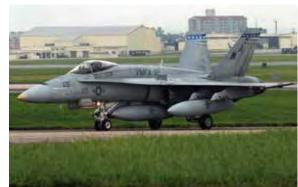
FA-18 A+ Hornet The FA-18 Hornet is an all-weather, supersonic aircraft used as an attack aircraft as well as a fighter. In its fighter mode, the FA-18 is primarily used as a fighter escort, for reconnaissance, and for fleet air defense; in its attack mode, the FA-18 is used for force projection, interdiction, and close and deep air support. MAG-41 (VMFA-112) currently
