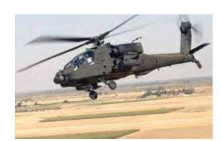
AH-64D Apache The AH-64D Apache is a four-blade, rotary-wing, twin-engine, attack aircraft with a tandem cocknit for a crew of two. The multi-mission AH-64D Apache Longbow is the next generation of the original AH-64A Apache. This aircraft is periodically stationed at NAS Fort Worth JRB on a temporary basis for maintenance with the U.S. Army Reserve, B Company, 90th Aviation Support Battalion.
