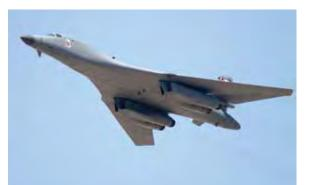
**B-1 Lancer** The B-1 is a long-range, multi-role strategic bomber for the Air Force. This aircraft carries the largest payload in the Air Force's long-range bomber fleet and can rapidly deliver massive quantities of precision and non-precision weapons against any adversary, anywhere in the world, at any time.
