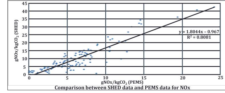
Measured NOx emissions from SHED more comparable to PEMS than from opacity testing and PM filter sampling
