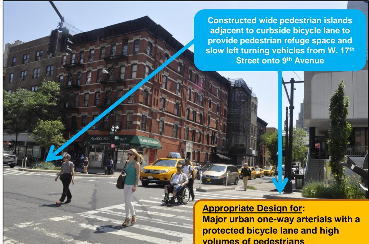
Constructed wide pedestrian islands adjacent to curbside bicycle lane to provide pedestrian refuge space and slow left turning vehicles from W. 17<sup>th</sup> Street onto 9<sup>th</sup> Avenue
