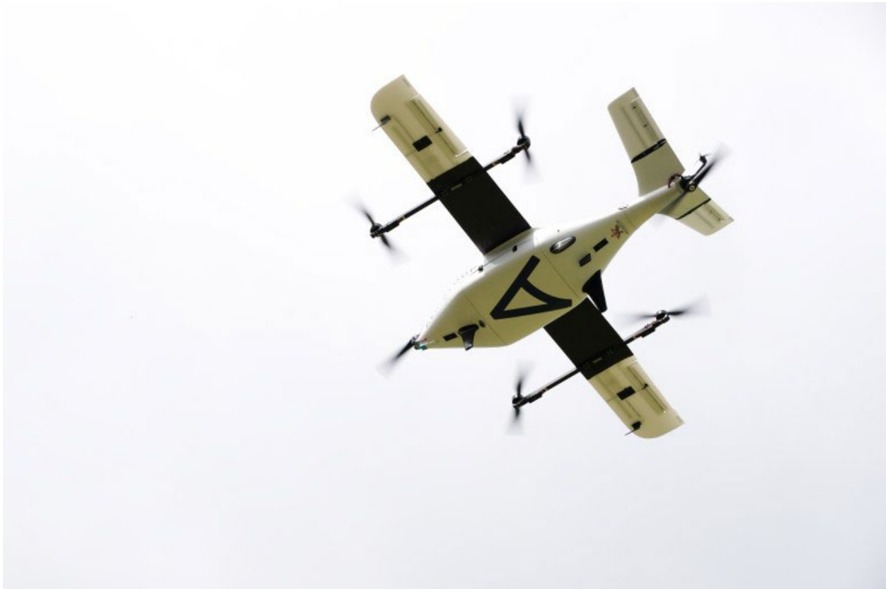
Aerialloop's ALT6-4 VTOL Delivery Drone is 6 feet long, battery powered and capable of carrying almost 9 pounds. (Camilo Diaz | Fort Worth Report)
