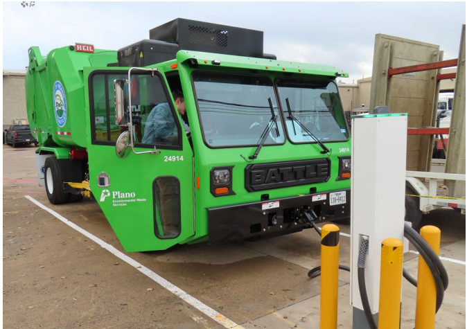
All-Electric Refuse Truck & Charger
