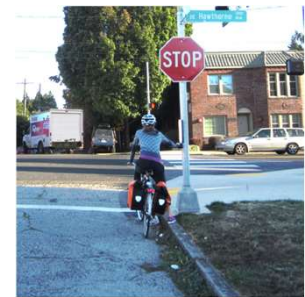
Figure 10-13: Example of Curbside Bicycle Pushbutton
