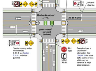
Figure 8-11: Example of a Median Used to Divert Traffic at a Major Street Crossing
