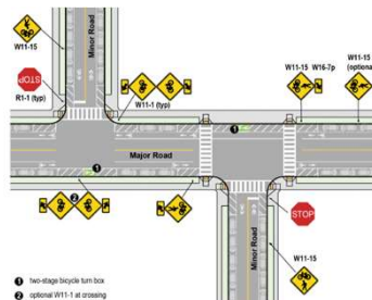
Figure 8-16: Example of Connecting Offset Bicycle Boulevard Segments Using a Blue Lane and Two-Stage Bicycle Turn Boxes
