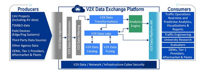
The V2X DEP supports data analytics engines with the data collected and uses other services such as a Security Credentials Management System (SCMS) to support trusted data exchange. The purpose of the V2X DEP is to:
