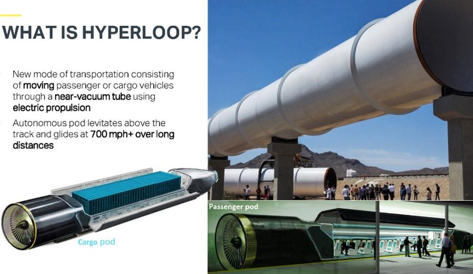
The image is a composite. On the left, a 3D cutaway of a 'Cargo pod' is shown, revealing internal components like a battery pack and a propeller. On the right, a large photograph shows a massive, white, cylindrical hyperloop tube structure supported by concrete pillars in a desert landscape. Below this, a smaller 3D rendering of a 'Passenger pod' is shown, which is sleek and aerodynamic with a large propeller at the front.
