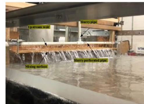
UTA Engineered Media for Biofiltration Swales BGG Round 3 Award (2021) Image courtesy of University of Texas-Arlington
