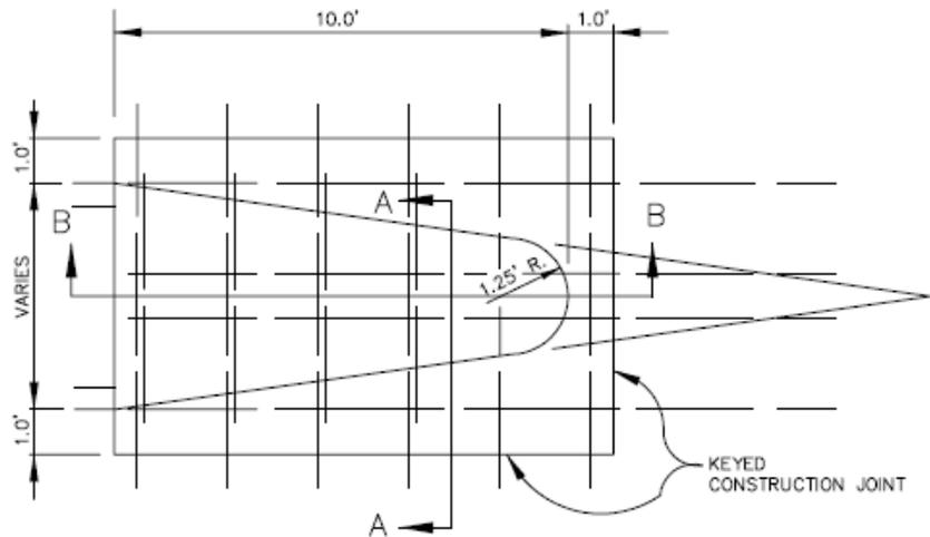
Low profile MONOLITHIC CONCRETE MEDIAN NOSE
