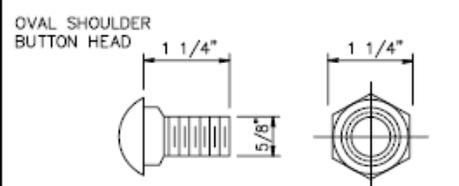
**ANCHOR OR SPLICE BOLT 5/8" NUT**
