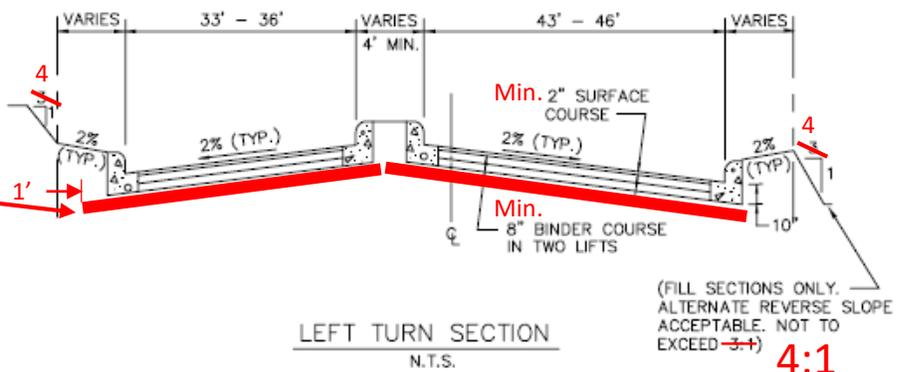
MIN. PAVEMENT DEPTH = 10"  $\left\{ \begin{array}{l} 2" \text{ HMA SURFACE COURSE} \\ 8" \text{ HMA BINDER COURSE} \end{array} \right.$
