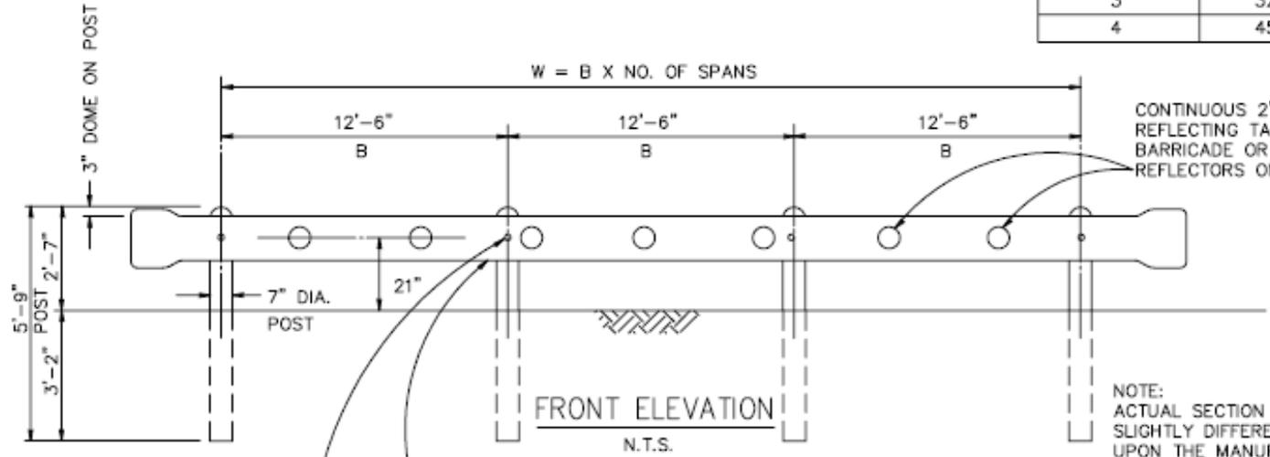
CONTINUOUS 2" RED REFLECTING TAPE ACROSS BARRICADE OR 4" DIA. REFLECTORS ON 5' CENTERS.
