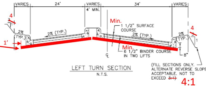
MIN. PAVEMENT DEPTH = 8" { 1 1/2" HMA SURFACE COURSE
