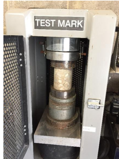
Concrete Strength Test
