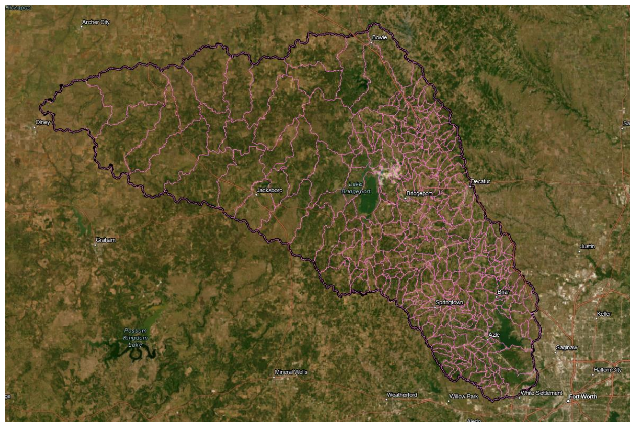
Figure 3-2. HEC-HMS Final Subbasin Delineation for TSI West Fork of the Trinity River Area.
