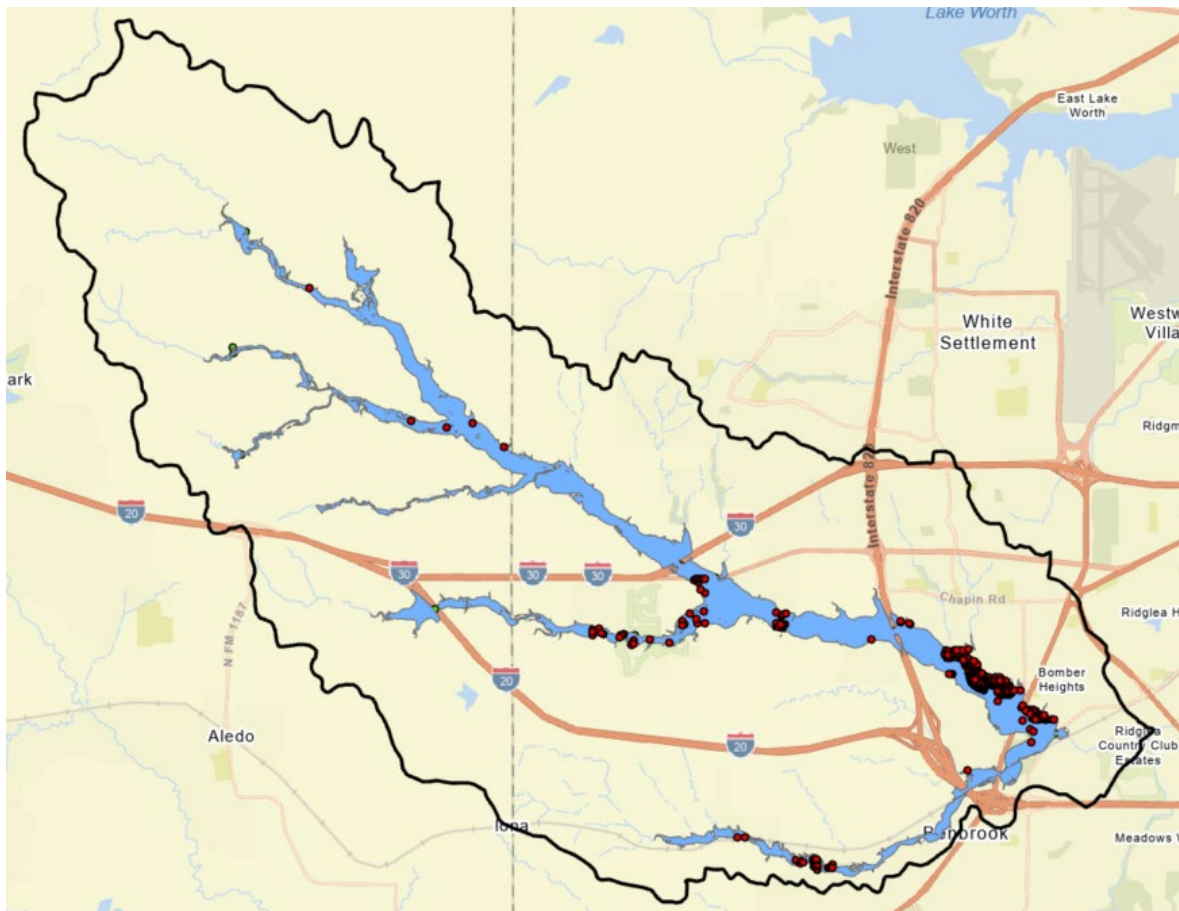
Figure 3-1. Existing Conditions, 100-year Flooding in 2020
