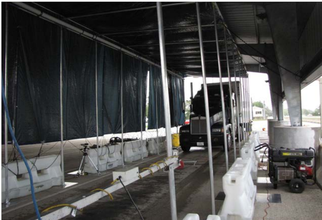
Figure 7: SHED Testing Setup: (Top) NWWS Shed and (Bottom) Sampling Tent in Lane 1.
