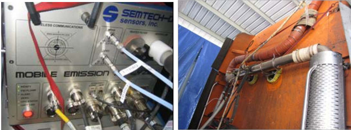
Figure 10: SEMTECH-DS (Left) and EFM Installed on a Test Vehicle (Right).
