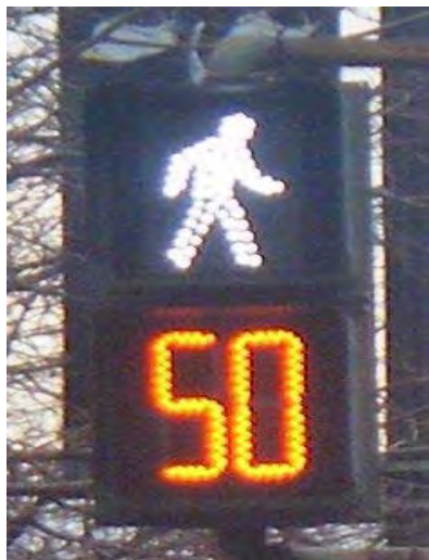
Pedestrian countdown signal - Dallas, TX Source: NCTCOG
