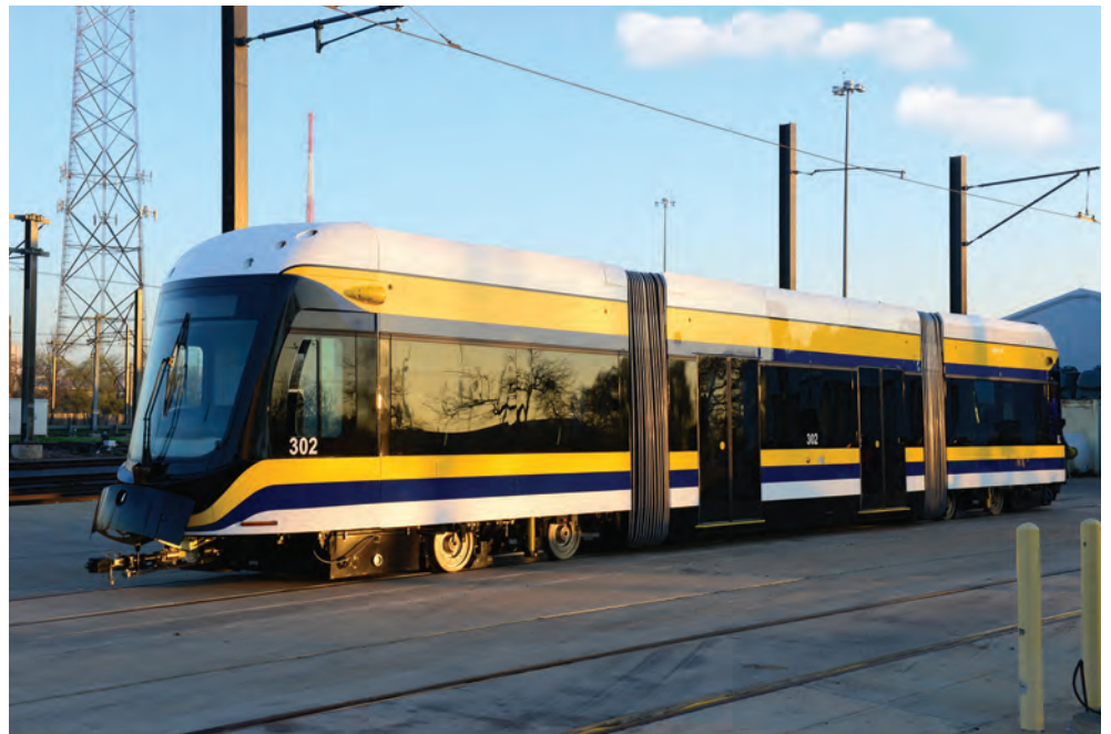
The Dallas Streetcar vehicles, designed and built by Brookville Equipment Corp. of Pennsylvania, will be the first dual-mode streetcars built in the U.S.
