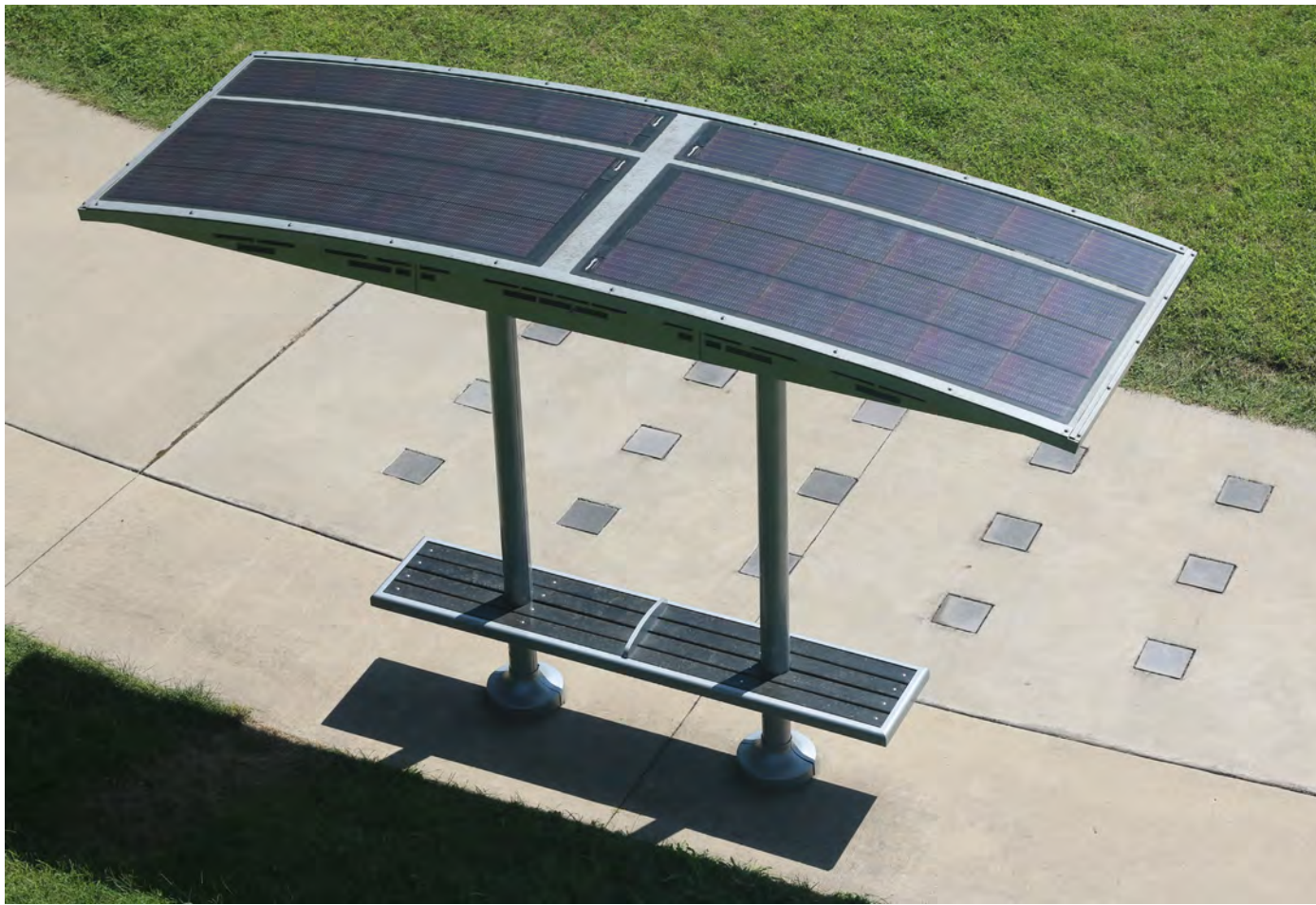
Above: Solar panels providing shade at a bus stop.
