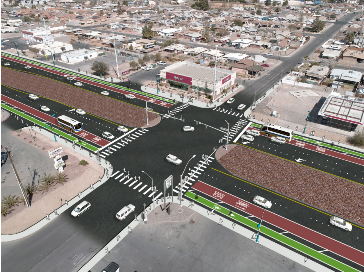
Rendering of Boulder Highway after conversion to a complete street. Rendering courtesy of the city of Henderson, Nevada.
