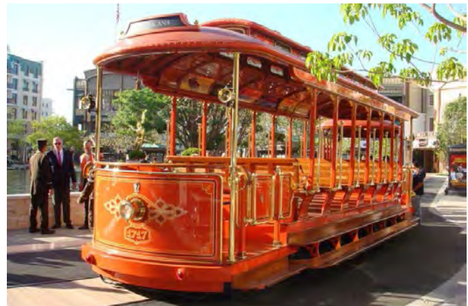
An example of a replica streetcar that is battery-powered. Image source: www.triplannermag.com
