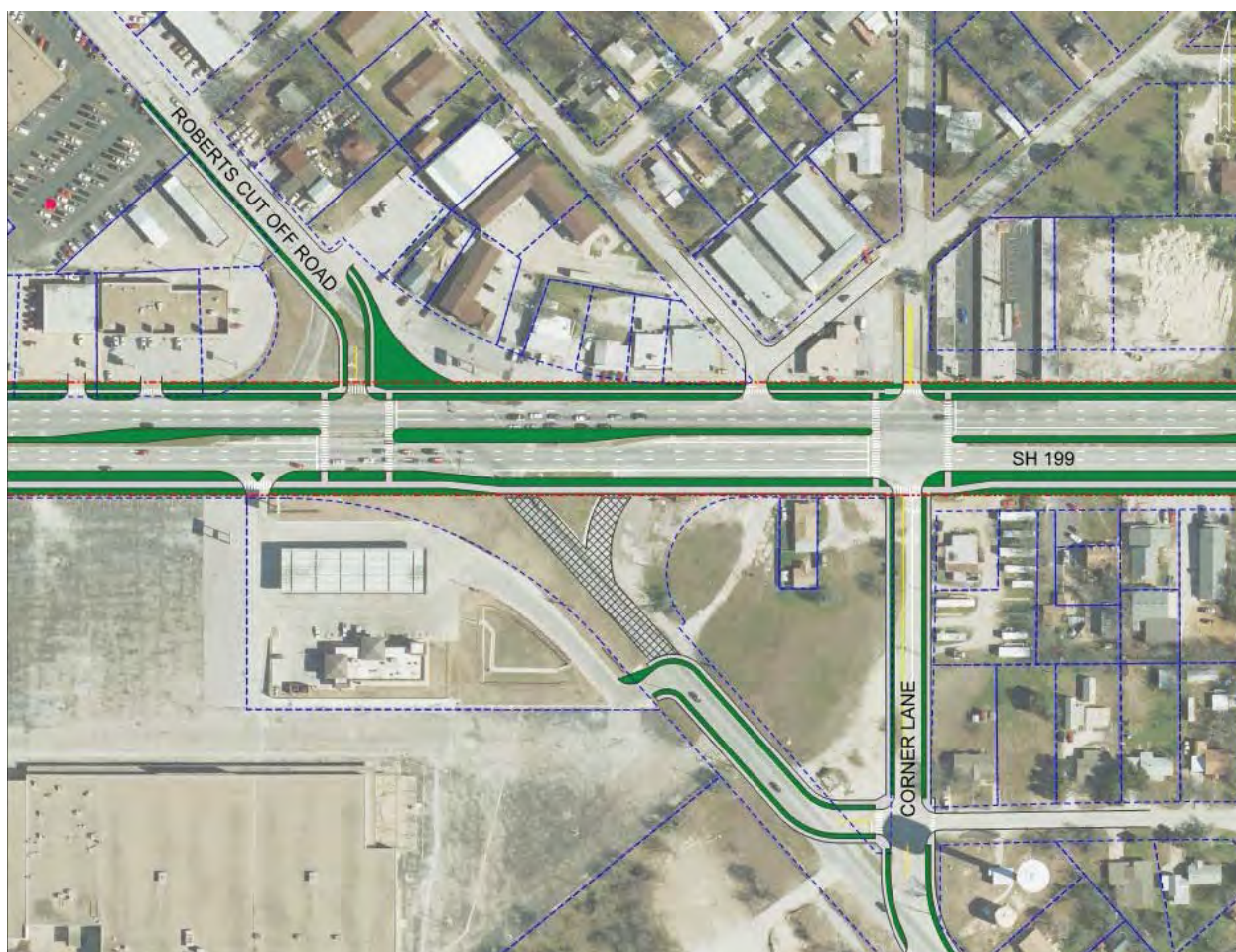
Figure 11. Alternative Intersection Geometry – Roberts Cut Off Road
