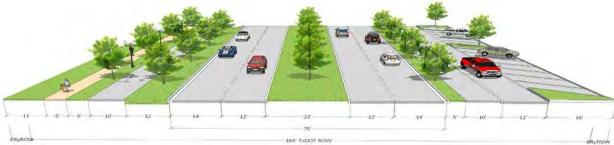
Figure 3. SH 183 Context Zone 3 Proposed Street Section
