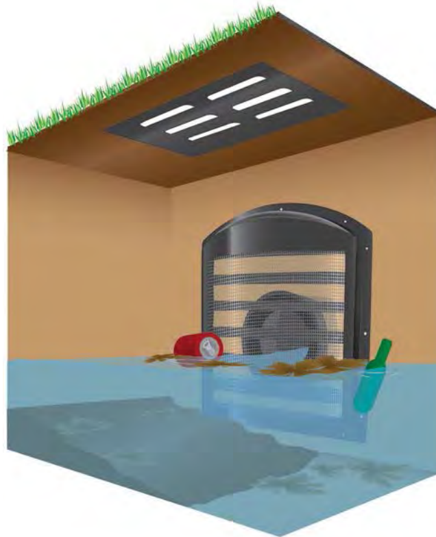
Figure 4. Inlet Screen Inside Catch Basin
