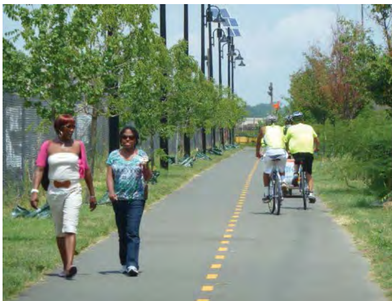
Figure 7. Enhanced Sidewalk with Centerline Striping
