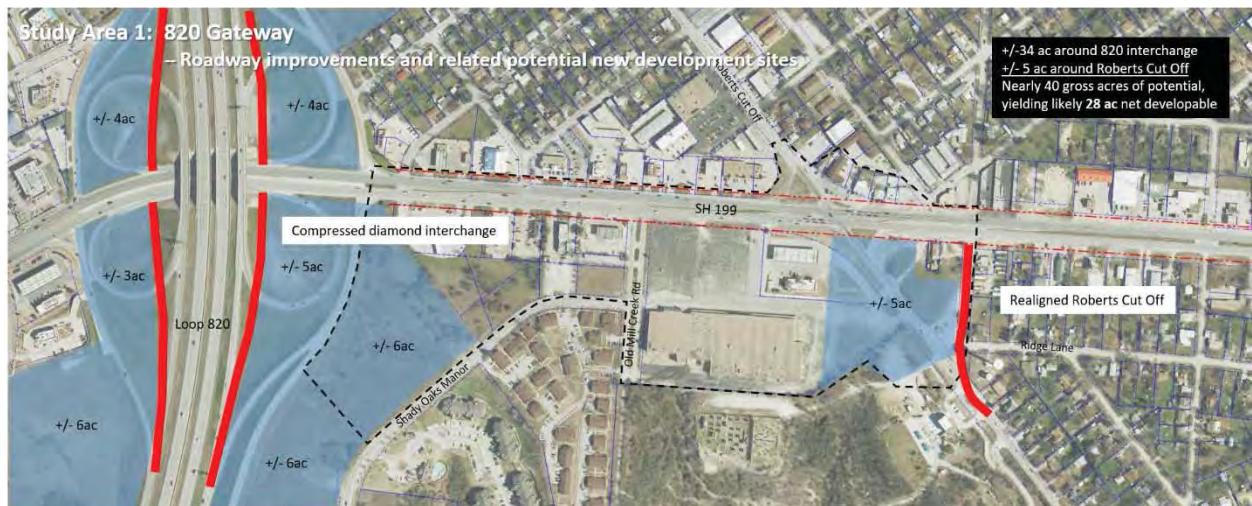
Figure 24. IH 820 Gateway: Roadway Improvements
