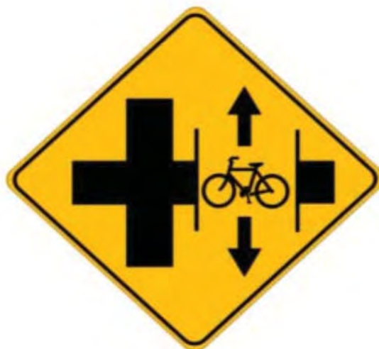
Figure 30. Adjacent Path Sign
