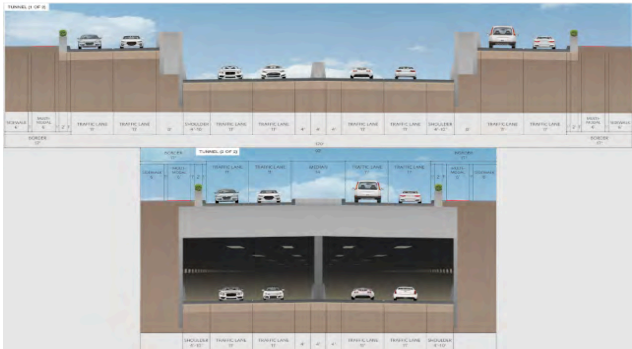
Cross-section of possible tunnel options (top: Only a century to get a park on it)
