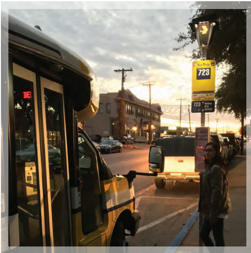
In the Bishop Arts District, a solar-powered light tops the bus stop pole to brighten the area and draw the bus operator’s attention to waiting customers.
