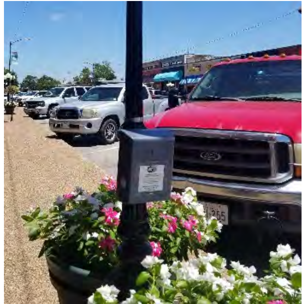
Photo of automatic counter used in pedestrian count
