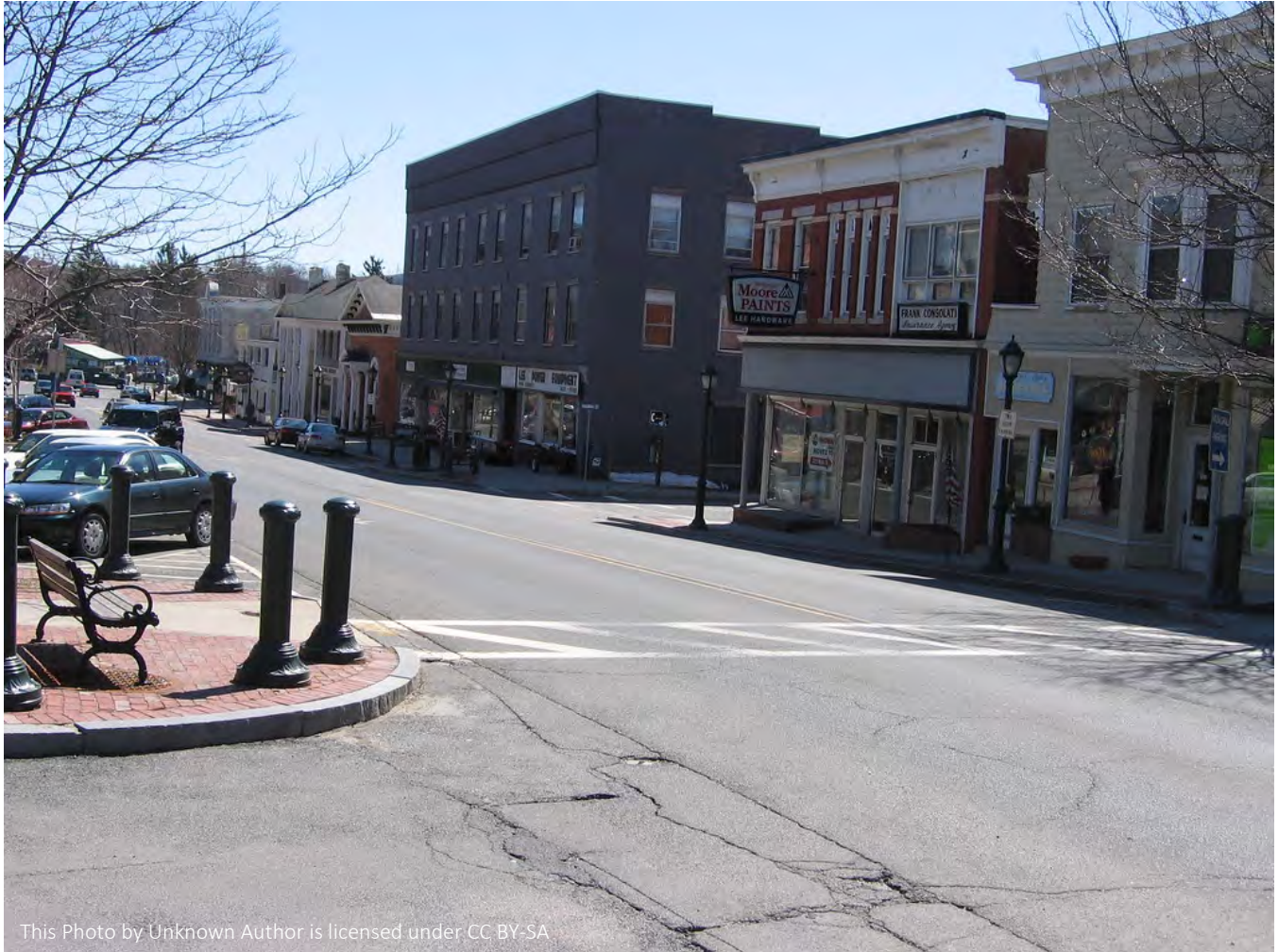
Figure 9: Curb Extension Example
