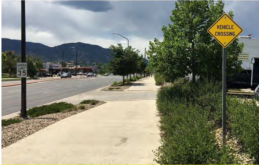
Figure 27. Signage to Warn People Walking and Biking on Enhanced Sidewalk of Potential Cross Traffic at Driveway
