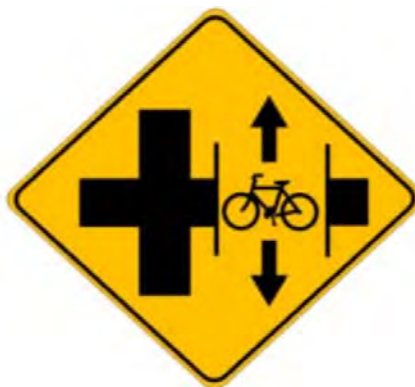
Figure 26. Adjacent Path Sign
