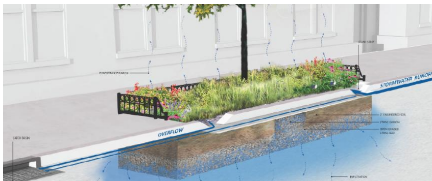
Figure 68. Isometric view of a New York City right-of-way bioswale. Source: NYC Department of Environmental Protection.
