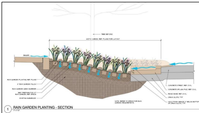
Figure 33. Plan of rain garden planting for the Elm Street streetscape improvements. Source: CCA Landscape Architects.
