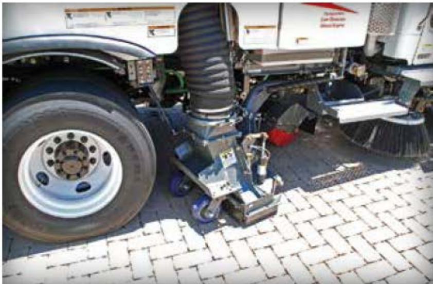
Figure 22. A true vacuum machine cleaning neglected PICP.
