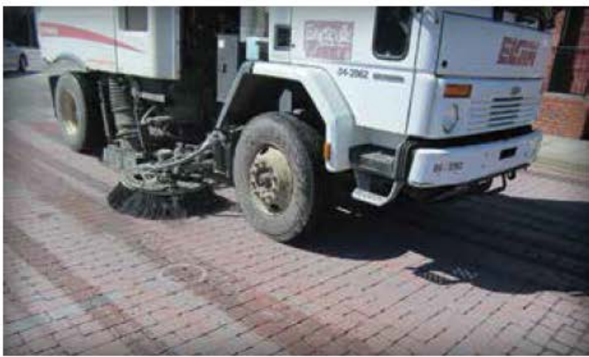
Figure 21. A regenerative air machine cleaning a PICP parking lot.
